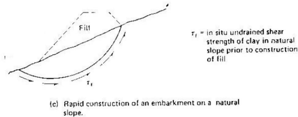
Fig. 11.37 Some examples of CU analyses for clays (after Ladd, 1971b).
